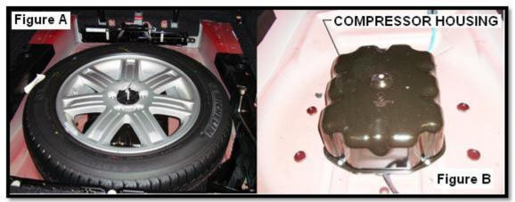
**3.** Remove cover from housing to expose the compressor (Cover is held on with the same mounting bolts that hold the compressor housing to the vehicle) (Figure C).
